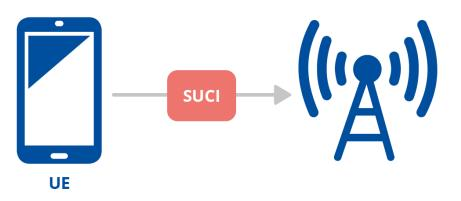
The subscription temporary identifier is called Globally Unique Temporary UE Identity (GUTI) which is sent to a user equipment after a successful activation of non-access stratum security. The Subscription Identifier De-Concealing Function (SIDF) is responsible for de-concealing the SUPI from the SUCI. Only a network element of the home network can request SIDF.
