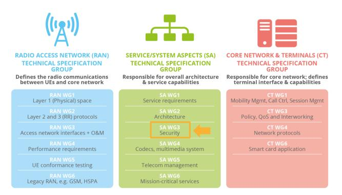
The main active working group addressing 5G security and privacy issues is 3GPP SA3<sup>12</sup>. The group is responsible for identifying the security and privacy requirements and defining the security architectures and associated protocols to address these requirements. 3GPP SA3 also ensures that cryptographic algorithms which need to be part of the 5G security specifications are available.
